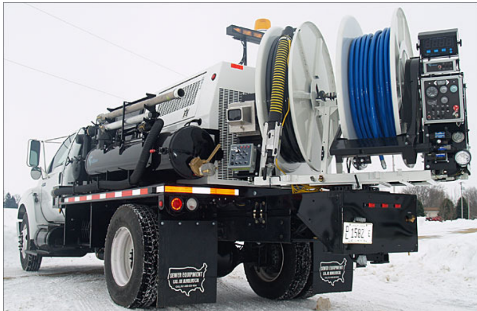
The Model 747-TK offers our most popular truck jet features (Rotating Hose Reel, Duraprolene Water Tank, Triplex Water Pump) as well as full length tool trays and deck mounted lateral hose reels.
